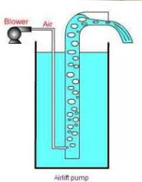
**Airlift Pumps.** This generic illustration shows the mechanics of the "airlift pumps" used in this system, which are simple pipe conduits through which pressurized air (from blower) is introduced at the bottom and by fluid pressure, water is carried up the pipe by ascending bubbles.
