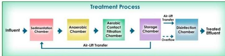
**Two Air Lift Pumps.** One Recirculating Air Lift pump sending process water and solids back to Chamber 1, and one Effluent Air Lift Pump for measured discharge of treated effluent. (See airlift pump info below).
