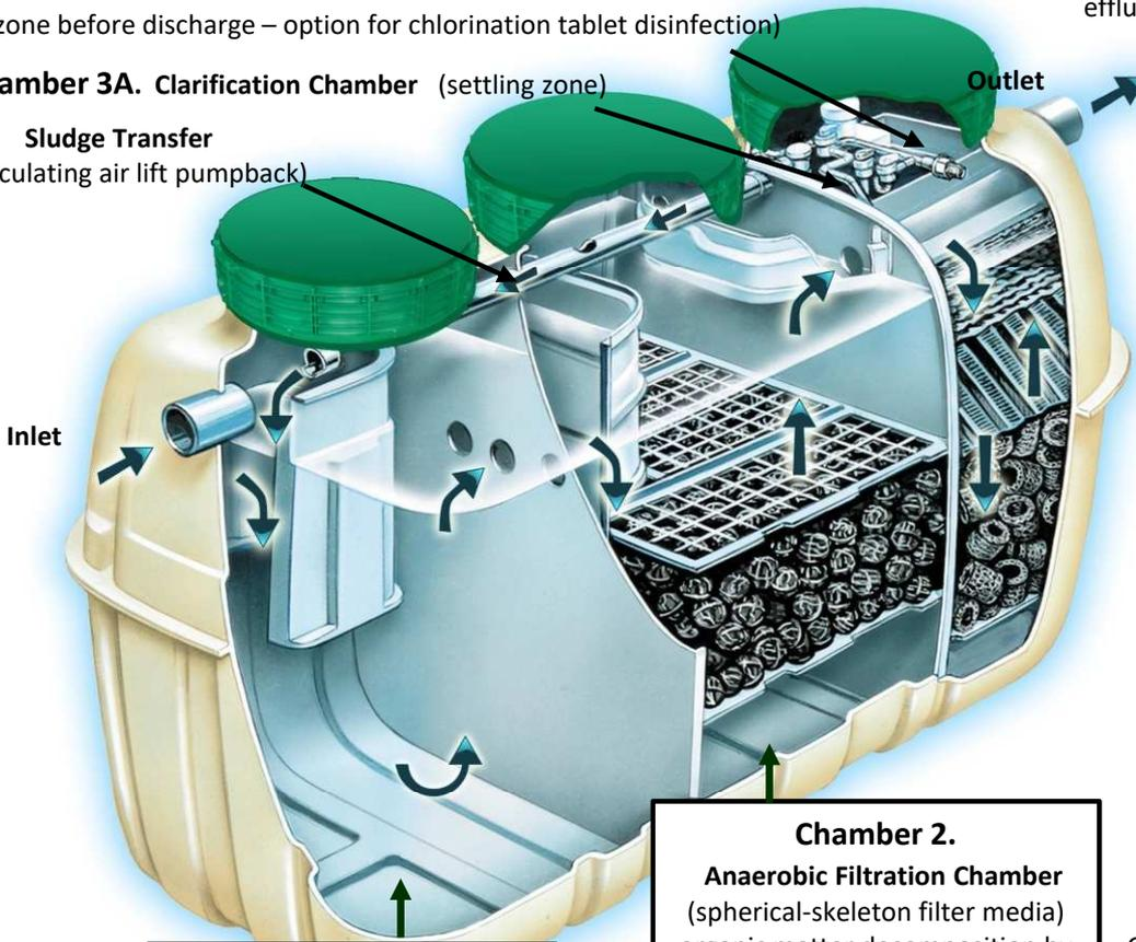
**Chamber 1. Sedimentation Chamber**
