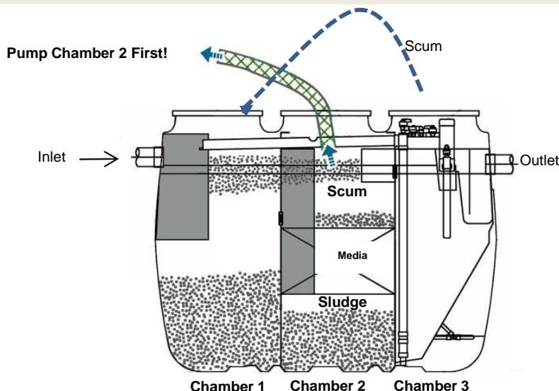
**Step 3. With pumpout hose, remove scum and sludge on the filtration media from Chamber 2**
