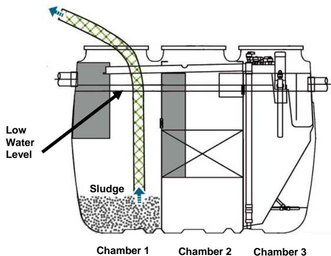
**Step 5. Remove scum and sludge Chamber 1.**
