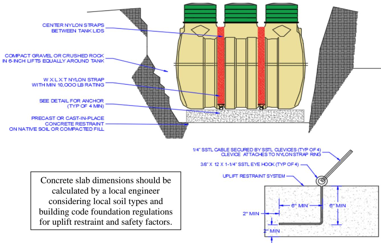
Figure 7 – Concrete Slab Approach for Uplift Restraint
