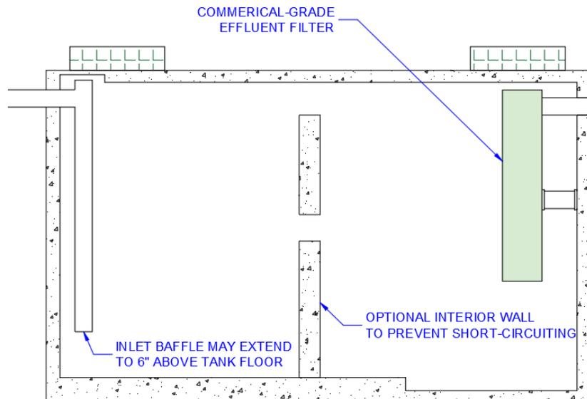
**Figure 5—Grease Trap**
