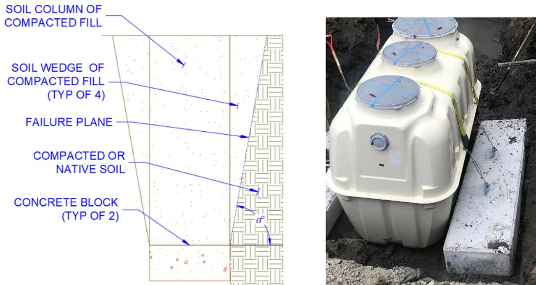
Figure 6 - Soil Wedge Approach for Uplift Restraint
